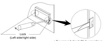
Unlock using such an screwdriver. Gently press outside on handle. • Recommended tool: Blade screwdriver
