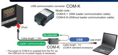
The RB series has a standard loader port to connect to a PC USB port via COM-K (USB communication converter). Using Win-UCI software on the PC, parameter settings can be easily saved on the PC in CSV format, and the same parameter settings are easily copied to other controllers.
