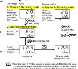
1\_Manipulated output value (MV) can be displayed on the MV display unit (third display unit). Similarly, while the Input 2\_ PV/SV monitor is displayed on FZ400/900, the Input 2\_Manipulated output value (MV) can be displayed on the MV display unit (third display unit). These parameters are set in H: Engineering mode.
