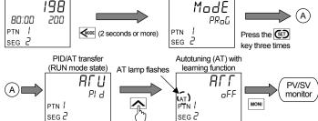
If set to PI by pressing the UP key, the AT starts. At this time, the AT lamp flashes.
