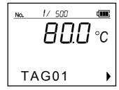
2. Press the ▲ or ▼ key while displaying the display memory screen to display the screen to be deleted.
