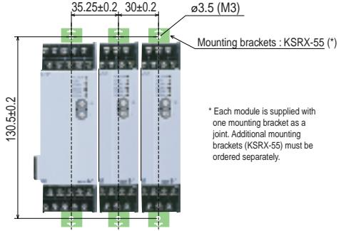
\* Each module is supplied with one mounting bracket as a joint. Additional mounting brackets (KSRX-55) must be ordered separately.
