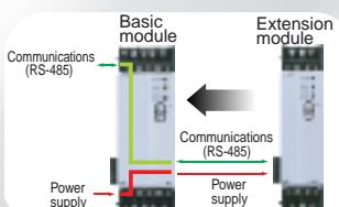
Communication and power supply for extension modules are just connecting modules.
