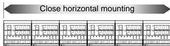
Six units maximum may be mounted together and maintain UL recognized, although it is possible to have more than six units.
